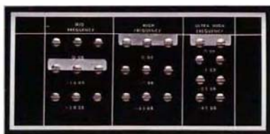
Level adjustments are made via bus bars.
